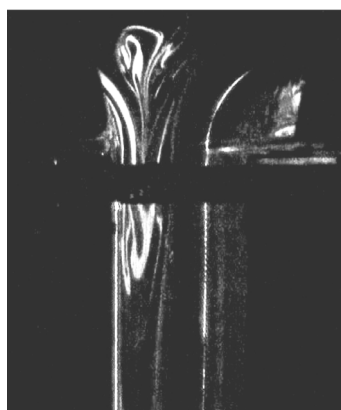
Fig. 5. Experimental device to generate natural convection flow in an air channel with the laser equipment, reverse flow visualization
