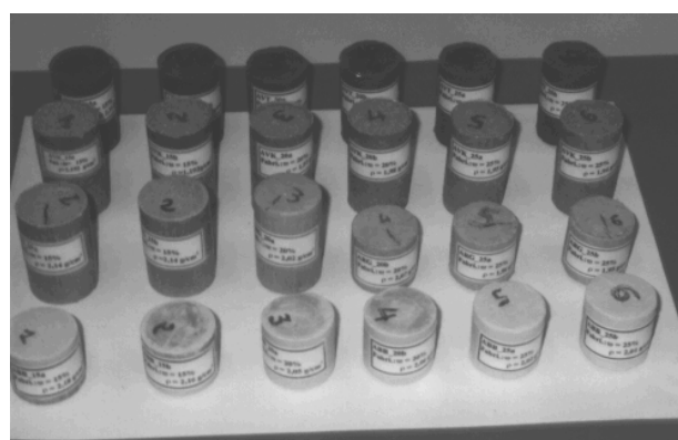
Fig. 3. Clay specimens with cylindrical shape (from front to the back: ABB, ARGK, AVTK, AVK clays)
