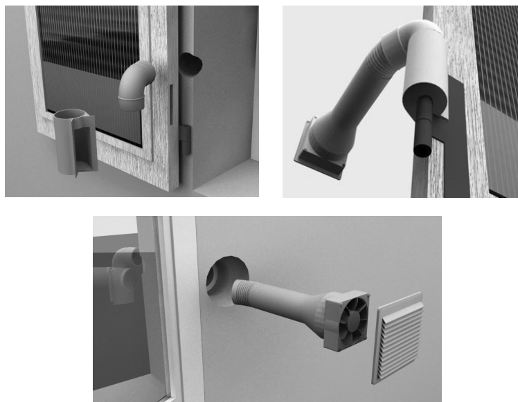
Fig. 4. Principle of the new solar air shutter and the air collector: the rotative part on the shutter, the fixed part in the wall and a view of inside house
