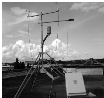
Fig. 2. Wind velocity and solar radiation measurement apparatus
