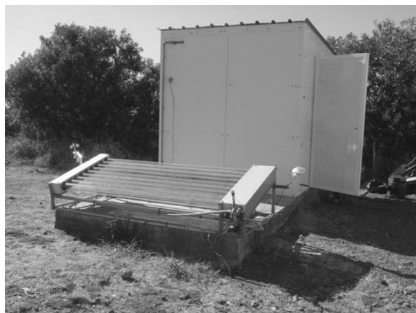
Solar collectors test bench according EN 12975-2
