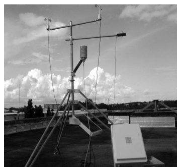
Fig. 2. Wind velocity and solar radiation measurement apparatus
