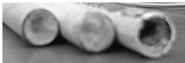
Fig. 2. Scale formation on the polypropylene conducts
