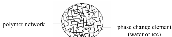
Fig. 1. Schematic representation of a spherical PCM particle
